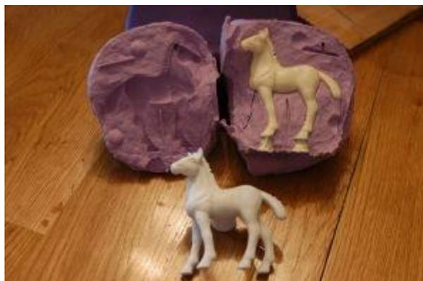
***A small silicon rubber mould to cast a small resin object.***
