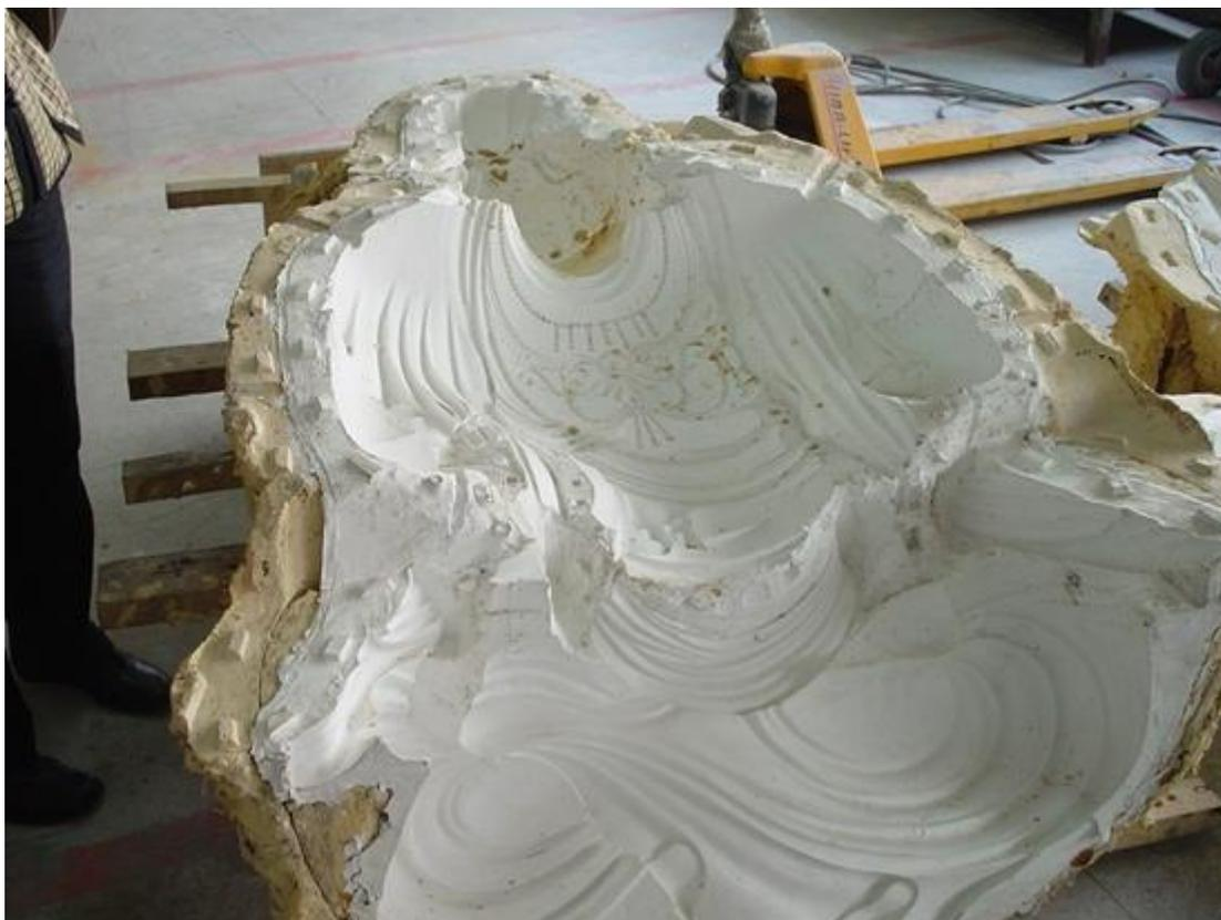
***A large silicon rubber mould half for casting a large resin object. There are intricate lines and contour in the rubber mould which would not be found in steel mould due to the draft angle.***
